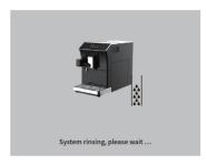
"Rinsing": start to rinse internal tubes and waste water will flow out of the coffee outlet after rinsing. The display interface is shown as the figure (dynamic display).
