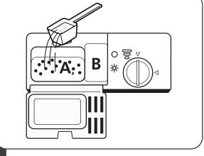
Add detergent into the larger cavity (A) for the main wash cycle. For more heavily soiled wash loads, also add some detergent into the smaller cavity (B) for the pre-wash cycle.
