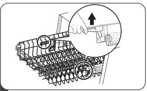
To lower the upper basket, lift the adjust handles on each side to release the basket and lower it to the lower position.
