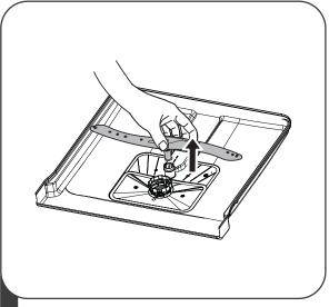
To remove the lower spray arm, pull out the spray arm upward.
