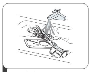
Larger food remnants can be cleaned by rinsing the filter under running water.
