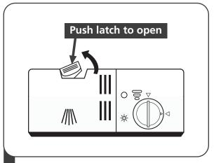
Press the release catch on the detergent dispenser to open the cover.
