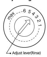
Turn the rinse aid indicator dial to a number between 1 and 6. The higher the number, the more rinse aid the dishwasher uses. If the dishes are not drying properly or are spotted, adjust the dial to the next higher number until your dishes are spot-free. Reduce it if there are sticky whitish stains on your dishes or a bluish film on glassware or knife blades.
